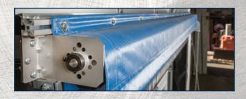
All doors come with a full width roll cover to protect the top roll assembly, while providing a tight seal for the industry's best insect control.
