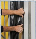
No fabric trimming on side seal panels for projection mount installations. Panels are preinstalled in the door track at the factory. The wall side of the panels are snapped into the wall mounted receiver.
